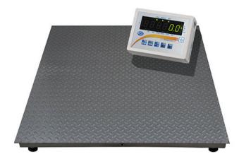
Approved - calibrated parcel scales up to 6,000 kg / Resolution from 0.1 kg/ Bidirectional RS-232 interface / Tare weight storable / Piece counting function/ Optional: analog output 4-20 mA, 0-10 V, OC switch contacts, etc.
